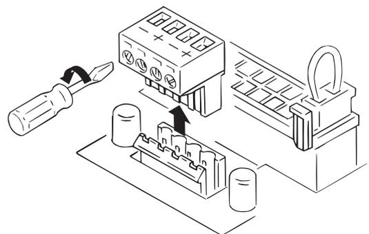
2-2. Insert the stripped cable ends into the input connector, and tighten the connector screws.
