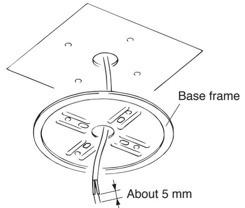
1-2. Secure the base frame to the wall or ceiling panel with screws at four places shown on the right.
