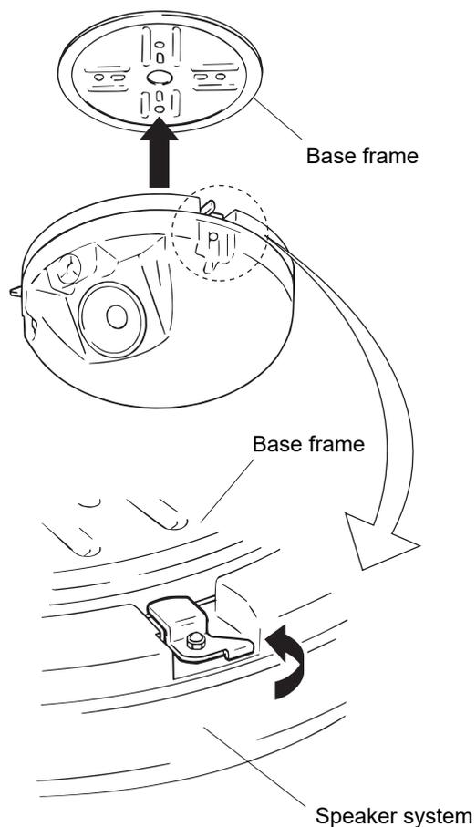
3-3. Position the speaker and tighten the three locking screws.
