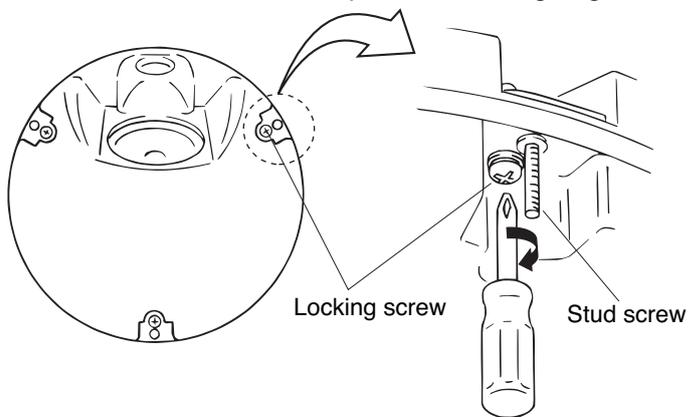
3-4. Set the front grille's aiming marker to the speaker front (i.e. speaker orientation) so that the three stud screws align with the corresponding stud receptacles, then push the grille onto the speaker.
