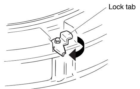
3-2. After aligning the speaker with the base frame, rotate the three lock tabs back into position to clamp the speaker to the base frame. (Temporary fixing state.)
