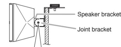
Refer to the figures below for the positional relationship between the speaker bracket's "groove" and the joint bracket's "indentation."
