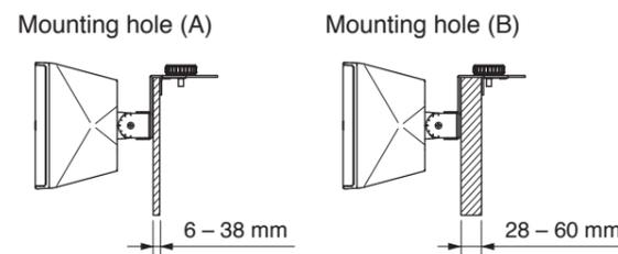
**Step 5.** Mount the speaker to the partition board. Slide the sliding bracket to pinch the partition board between the sliding bracket and hanger bracket, then tighten the knob bolt.
