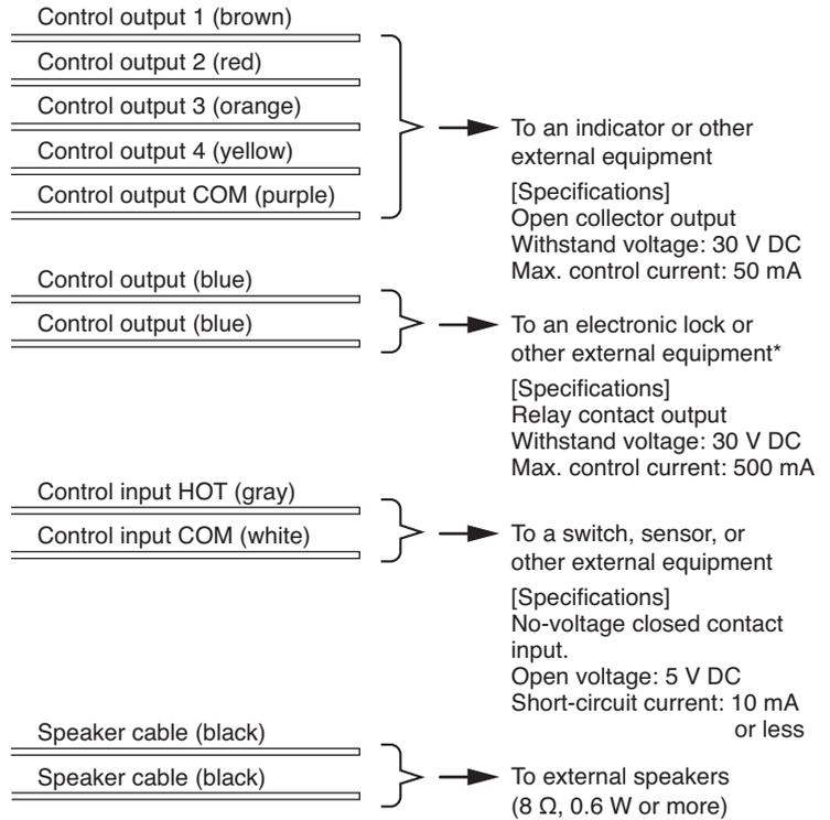
\* Connection example (When using a 24 V DC relay)
