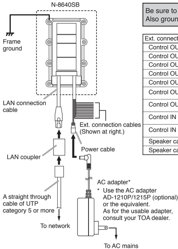
Be sure to ground the N-8640SB's frame ground terminal. Also ground the electrical box if used.
