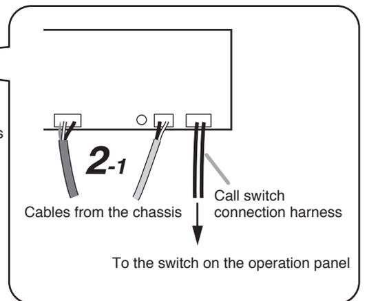
**Step 5.** Run the connection cables through the case's cable entry holes, then make cable connections.
