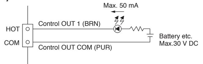
[Example 2] (When using a 24 V DC relay)
