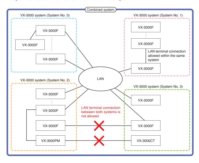
Direct connection without switching hub as shown below is not allowed as well.
