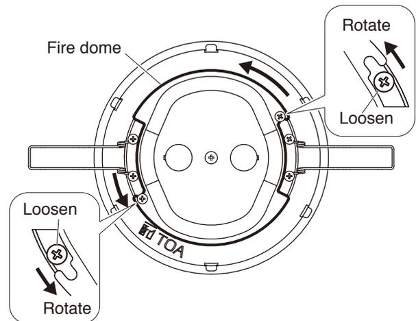
**Step 3.** Punch out the knockout hole in the fire dome, then install the supplied cable entry rubber grommet in the knockout hole.
