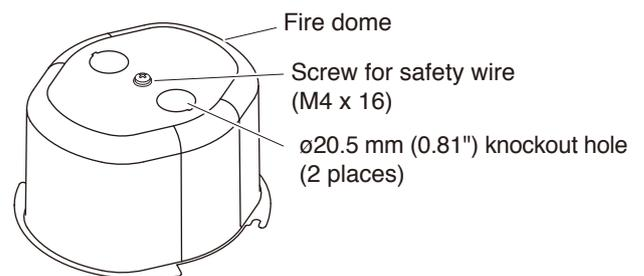
**Step 4.** Install the safety wire to the M4 screw on the top of the fire dome as needed.
