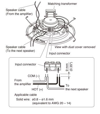
**4-2.** Change the input impedance as needed. The speaker's input is factory-preset to  $1.7 \text{ k}\Omega$ . When changing the input impedance, detach the black wire connected to the matching transformer, and reinsert it into the desired input tap referring to the table below.
