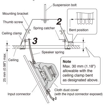
**Step 2.** Place the mounting bracket in the hole and secure it with the thumb screws in the two ceiling clamps. **Note**
