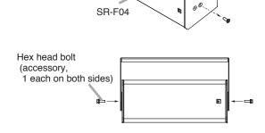
**Step 3.** Attach this bracket to the Bracket B of the speaker mounting bracket to join.
