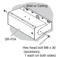
**Step 4.** Loosen the hex head bolts installed in **Step 3**, and adjust the vertical angle of the SR-F04. Then, securely retighten the bolts.
