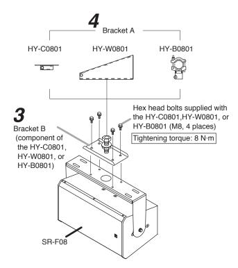
**Step 5.** Loosen the hex head bolts installed in **Step 2**, and adjust the vertical angle of the SR-F08. Then, securely retighten the bolts.
