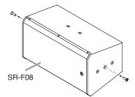
Step 2. Install this bracket to the wall or ceiling.
