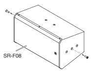
**Step 2.** Attach the bracket to the SR-F08 with the supplied hex head bolts.
