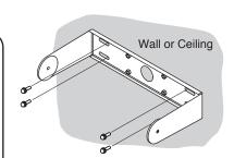
Secure the bracket with 4 bolts using all the 4 mounting holes. For the mounting bracket's dimensions and the mounting hole positions, see "DIMENSIONAL DIAGRAM."
