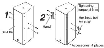
Attach the hand bracket aligning its curved line with the SR-F04's front direction.
