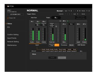
Click the screen name in the menu bar located at the left side of the browser screen to switch to the necessary screen. (See "SWITCHING THE SCREEN" on p. 7.)
