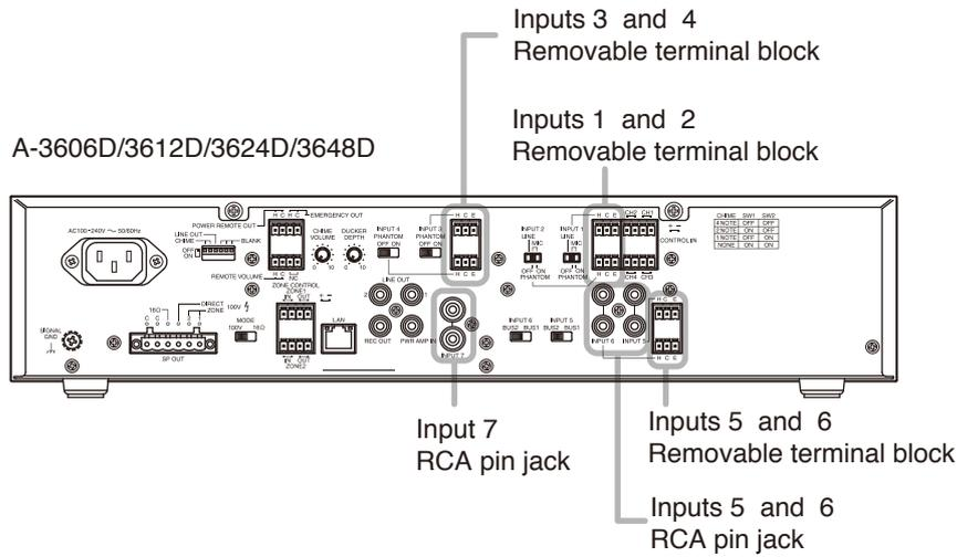
The terminal used for each of the Inputs 5 and 6 differs depending on the BUS setting switch (Refer to the next page.).
