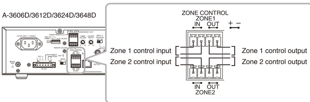
Control input signal specifications: Short-circuit current: 10 mA or less, open voltage: 35 V DC or less
