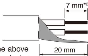
\*2 Expose 8 mm or more when using the above ferrule terminal, and cut off an extra conductor protruding from the sleeve.
