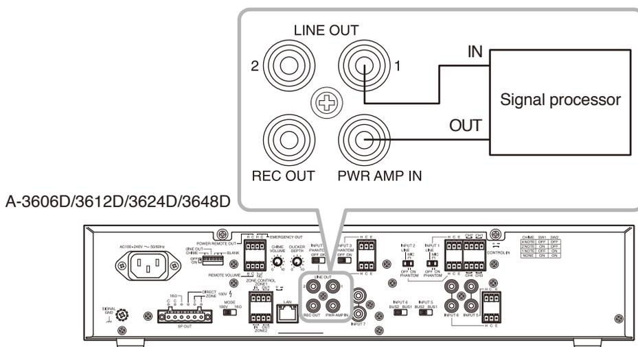
Line output specifications: 0 dB\*, 600 Ω, unbalanced, RCA pin jack
