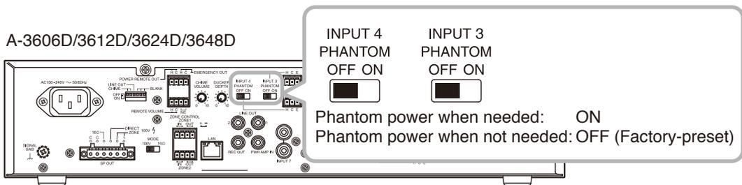
Input specifications: -60 dB\*, 600 Ω, electronically balanced
