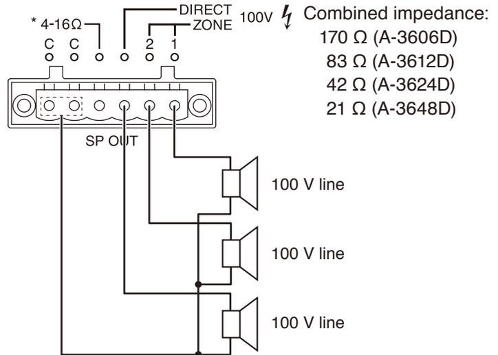
For the audio output at high impedance application setting, refer to "32. Output impedance setting switch" on p. 11.
