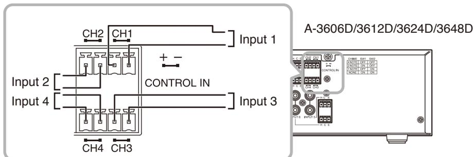
Input signal specifications: Short-circuit current: 10 mA or less, open voltage: 35 V DC or less
