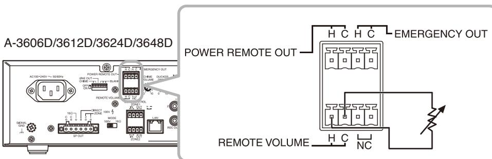
Connectable volume controller: 10 kΩ B-taper potentiometer
