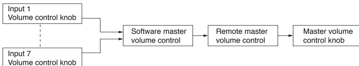
If any one of the volume controls is set to the minimum, no sound is output even if other volume control is set to the maximum. If you intend to adjust the volume value with the Software master volume control\*<sup>1</sup> or the Remote master volume control (see p. 15), adjust the volume value using the master volume control knob in advance. The value adjusted with the master volume control knob is the adjustable upper limit.
