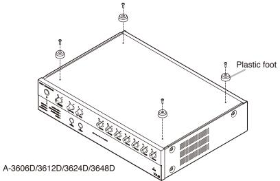
When installing the unit to an equipment rack, use the optional MB-25B Rack mounting bracket.
