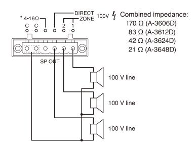
For the audio output at high impedance application setting, refer to "32. Output impedance setting switch" on p. 11.
