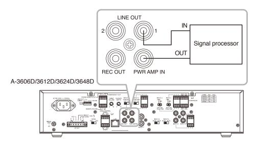
Line output specifications: 0 dB\*, 600  $\Omega$ , unbalanced, RCA pin jack Power amplifier input specifications: 0 dB\*, 600  $\Omega$ , unbalanced, RCA pin jack
