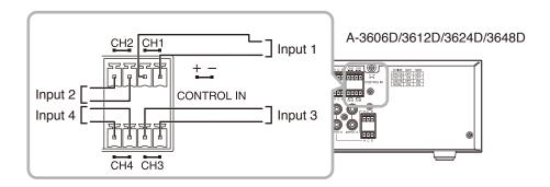
Input signal specifications: Short-circuit current: 10 mA or less, open voltage: 35 V DC or less
