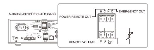
Connectable volume controller: 10 kΩ B-taper potentiometer
