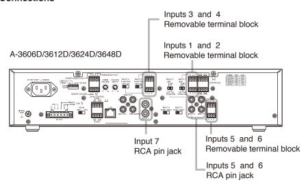
The terminal used for each of the Inputs 5 and 6 differs depending on the BUS setting switch (Refer to the next page.).
