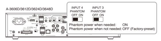
Input specifications: -60 dB\*, 600 Ω, electronically balanced
