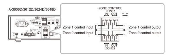
Control input signal specifications: Short-circuit current: 10 mA or less, open voltage: 35 V DC or less Control output signal specifications: Open collector output, withstand voltage: 30 V DC or less, current: 25 mA or less
