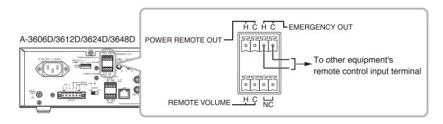
Output specifications: Open collector output, withstand voltage: 30 V DC or less, current: 25 mA or less
