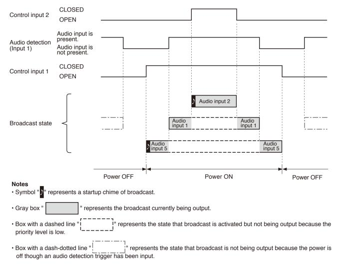
Only in the following case, the power is ON in the period that only the audio detection input is present. When the control input and the audio detection input with higher priority overlap, the power remains ON until the audio detection input is terminated after all control inputs are opened.
