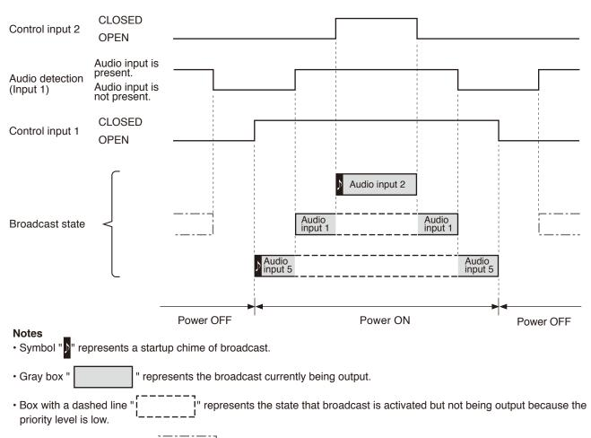
• Box with a dash-dotted line "\_\_\_\_\_\_" represents the state that broadcast is not being output because the power is off though an audio detection trigger has been input.
