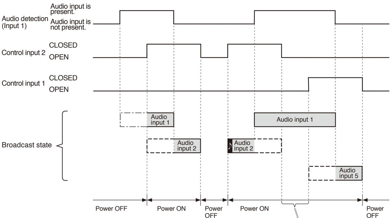
Even though the control input 2 is open, power remains ON because the audio detection (input 1) having higher priority than it is being kept.
