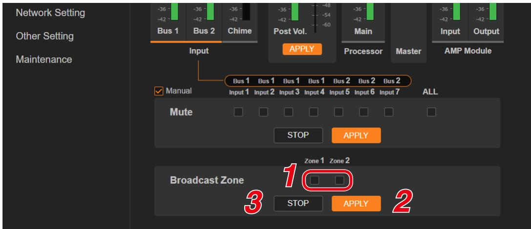
**Step 1.** Check the checkbox of the zone to select.
