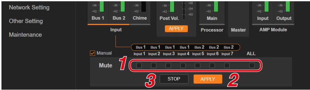
**Step 1.** Check the checkbox for the audio input to be muted.
