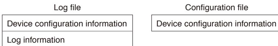
The log file consists of device configuration information and log information, and the configuration file consists of device configuration information only.
