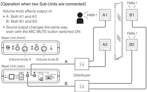
Note: Up to 3 Sub-Units each can be connected to A and B jacks.
