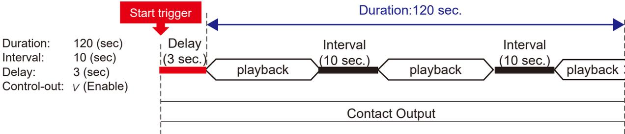
**[Controlling Start-to-Finish Duration When the Control Input Signal Mode is Set to Level ]**
