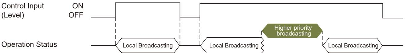
Local broadcasting continues as long as the Level signal is being received. If the broadcast is interrupted by a higher priority broadcast and the Level signal continues to be maintained when the higher priority broadcast ends, Local broadcasting will restart again.
