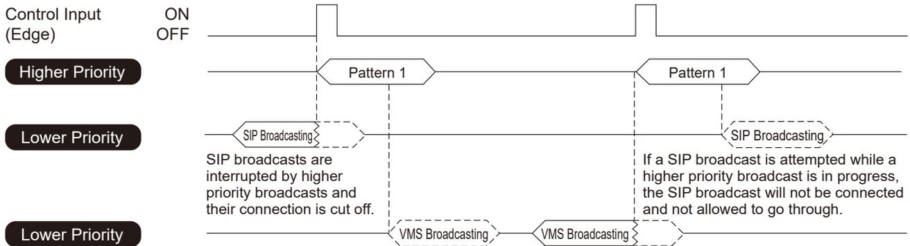
If a VMS broadcast is attempted while a higher priority broadcast is in progress, the VMS broadcast will not be connected and not allowed to go through.
