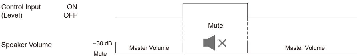
The speaker volume is muted while the Level signal is being received. The line output is also muted. Due to this, the audio volume control to be linked to the control input is made possible.
