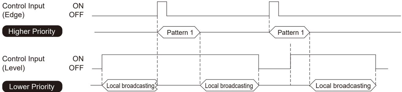
Lower priority Local broadcasts are stopped by higher priority broadcasts. If the Level signal input is maintained, the Local broadcasting will be restored after the higher priority broadcast ends.
