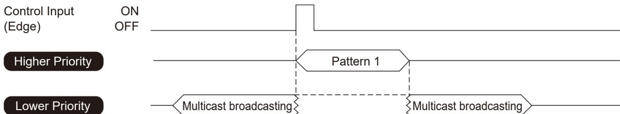
Lower priority Multicast broadcasts are stopped by higher priority broadcasts. If Multicast broadcasting packets have been received at the end of the higher priority broadcast, the Multicast broadcasting is restored.
