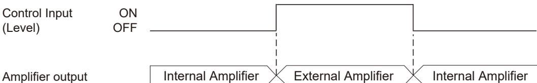
When a level signal is input, the external amplifier is enabled and its signal is output through the speakers. Switching between the internal amplifier and the external amplifier is carried out regardless of the operating status of the receiving device, except when the receiving device is in system mute mode.
