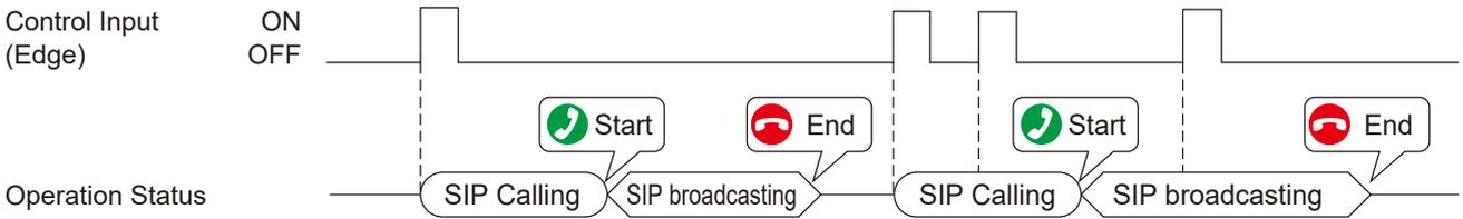
Makes a call to a SIP phone when the Edge signal is detected. Performing call reception at the call destination SIP phone causes the SIP broadcast to begin. When the SIP phone conversation is terminated, the SIP broadcast also ends. Even if the same event trigger is received during the SIP call or SIP broadcasting, the call or broadcast is not interrupted.
