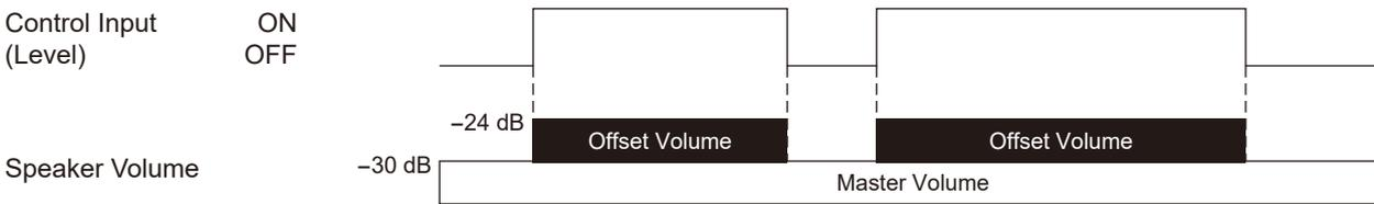
Offset Volume is applied while the Level signal is being received. Offset Volume is also applied to the audio of the ongoing broadcast in real time. This enables the audio volume control to be linked to the control input.
