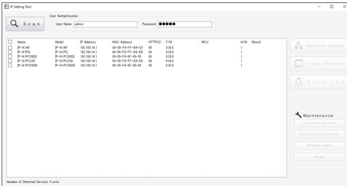
Selecting any device in the list by marking its corresponding checkbox activates its right-side button, thus making it possible to click on.
