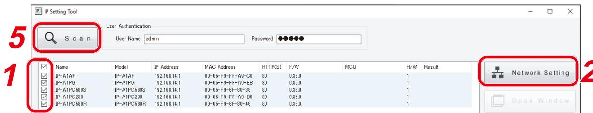
**Step 1.** Select the device(s) for which network settings will be performed by marking the corresponding checkbox in the Detection Results list.
